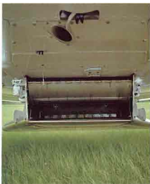
All purpose streamlined spreader, in stainless steel or aluminum, applies dry chemicals at rates from 5 to 200 lbs. per acre.
