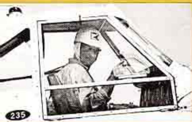
New storm windows on both sides add to comfort while taxiing, enable pilot to wipe off windshield from inside cockpit.
