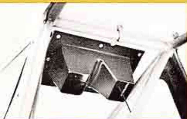
Three individually adjustable overhead vent locations for maximum comfort. Shown is new rear vent, which cools pilot's back and shoulders. Electric fan, mounted near floor, is now standard. The Mark 8 is optionally available for navigation and communications, with the speaker located in the headrest.
